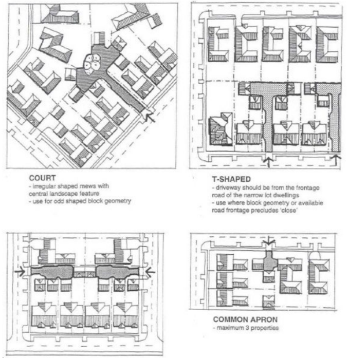
Figure E7.81: Shared Driveway - Design Principles
