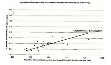
Figure 4 - Correlation of Bulk ECe (below 0.8m) and ECa (HCP) data
