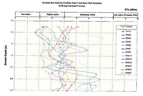
Figure 2c - "Mixed" Vertical Soil Salinity Profiles
