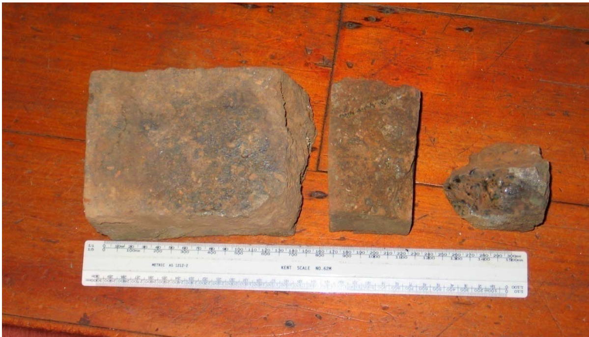
Figure 3.8: Three brick fragments recovered from Areas A and B. The central fragment is from Area B. Both the brick fragments from Area A had evidence of vitreous glaze, with notably the right fragment having glaze on the broken face indicating it probably exploded in the clamp kiln and the glaze then formed on the broken face.
