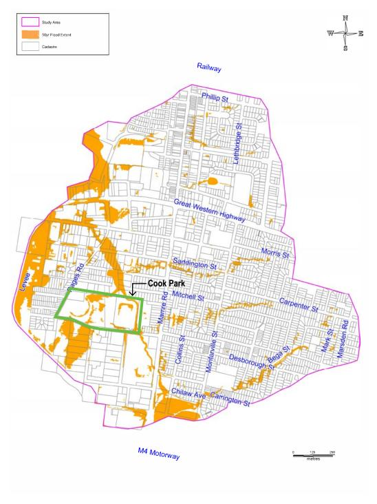
Figure 5f: 50 Year ARI - Flood Extend in Cook Park (Image from St Marys (Byrnes Creek) Catchment Detailed Overland Flow Flood Study - Final Report Prepared By Cardno)
