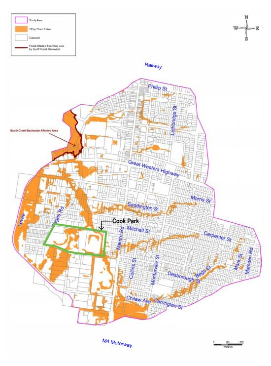
Figure 5e: 100 Year ARI - Flood Extend in Cook Park (Image from St Marys (Byrnes Creek) Catchment Detailed Overland Flow Flood Study - Final Report Prepared By Cardno)
