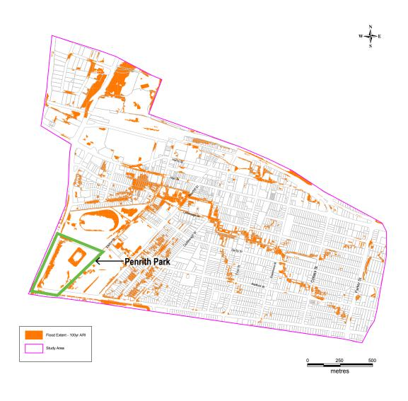
Figure 5c: 100 Year ARI - Flood Extend in Penrith Park (Image from Penrith CBD Detailed Overland Flow Flood Study - Final Report Prepared By Cardno)
