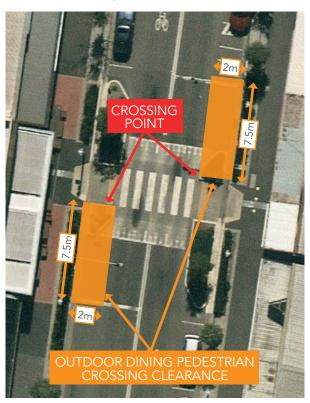
**Figure 3:** Minimum pedestrian crossing clearances when approaching a signalised pedestrian crossing
