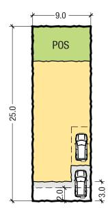
Example Built Form Typology Attached Front Loaded 9 x 25m (225sqm)
