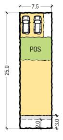
Example Built Form Typology Attached Rear Loaded 7.5 x 25m (187sqm)
