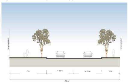
Figure E13.19 Secondary Street (without parking) - Type 2A
