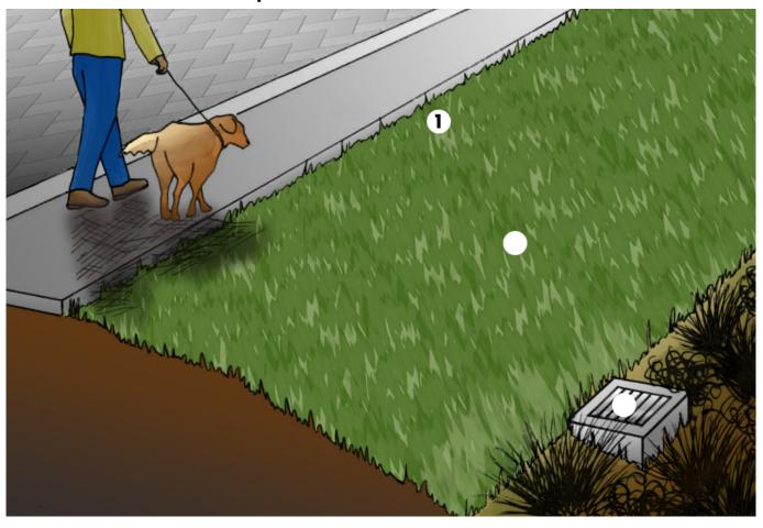
Figure 5: The functional components of a vegetated buffer strip.
