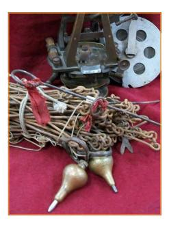
Throughout recorded history surveyors have used many devices for measuring distances. These devices have included rope, poles, grape vines, pacing, steel tapes, electronic devices and "chains". The basic "Gunter's" chain was the primary tool of surveyors to measure distance in North America from the 1600s to the end of the 1800s. The basic idea of a chain is to be 66' long with 100 links making up the chain.
