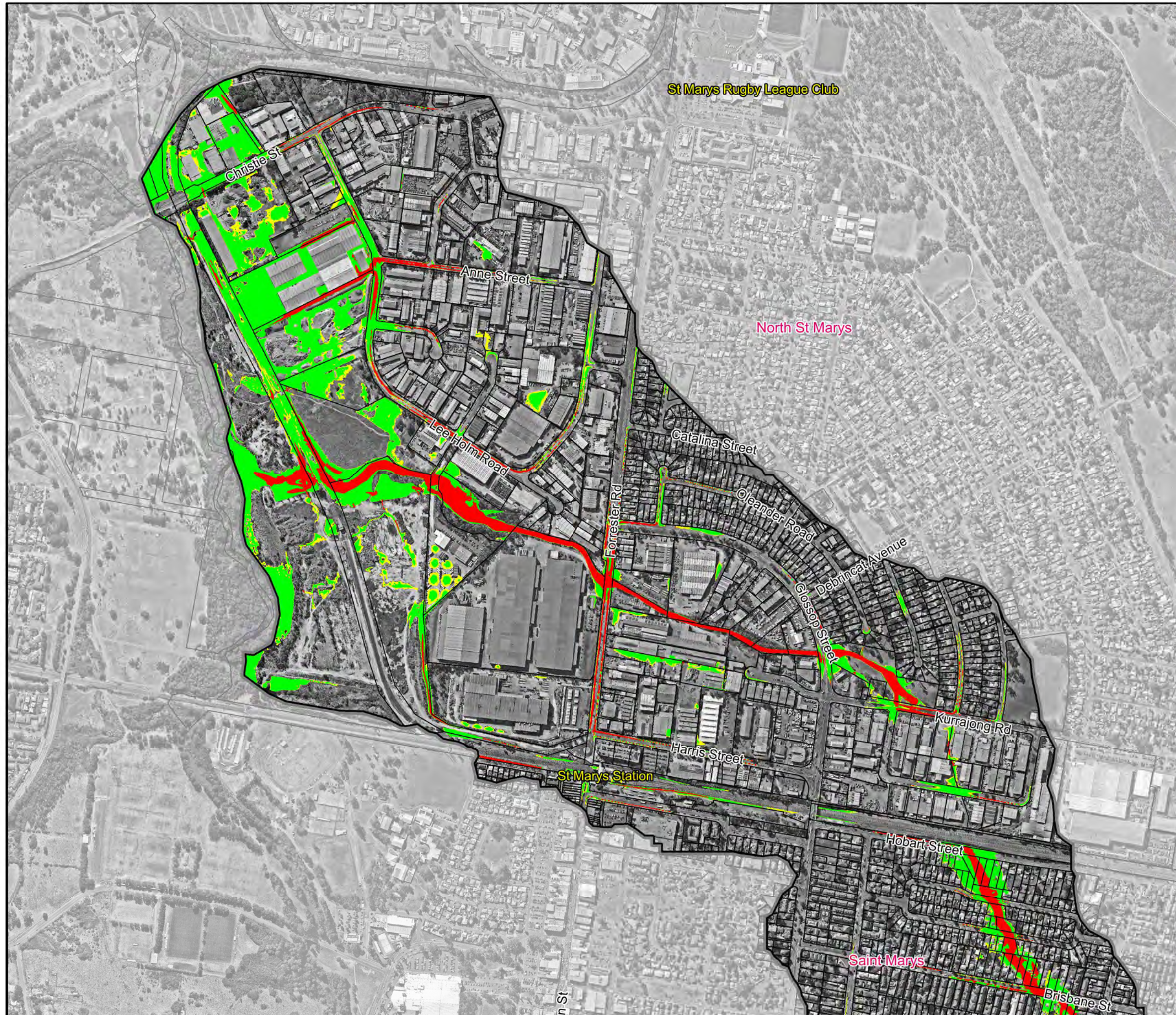
Figure 40.2 Hydraulic Categories for the 0.5%AEP
