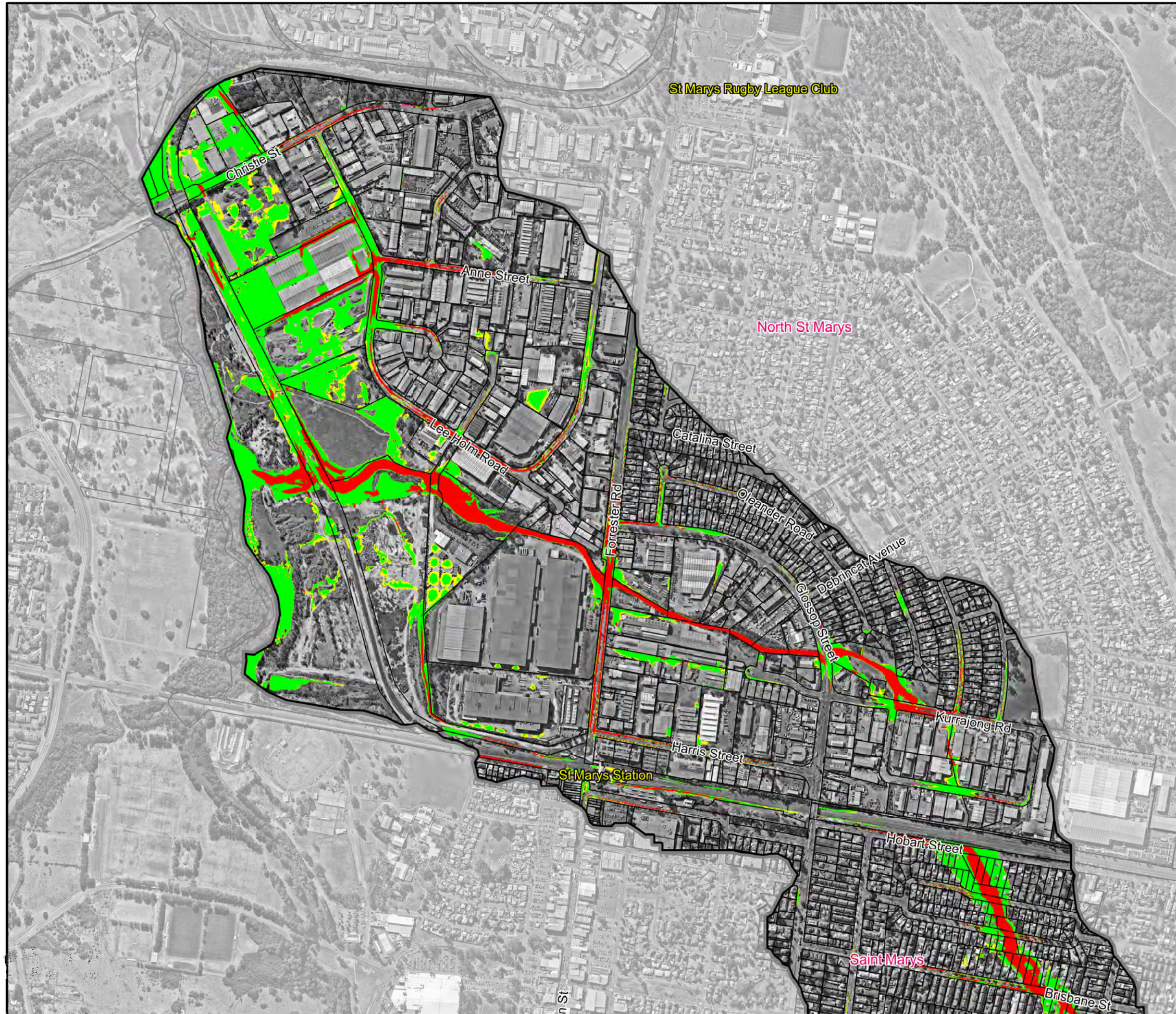
Figure 41.2 Hydraulic Categories for the 0.2%AEP
