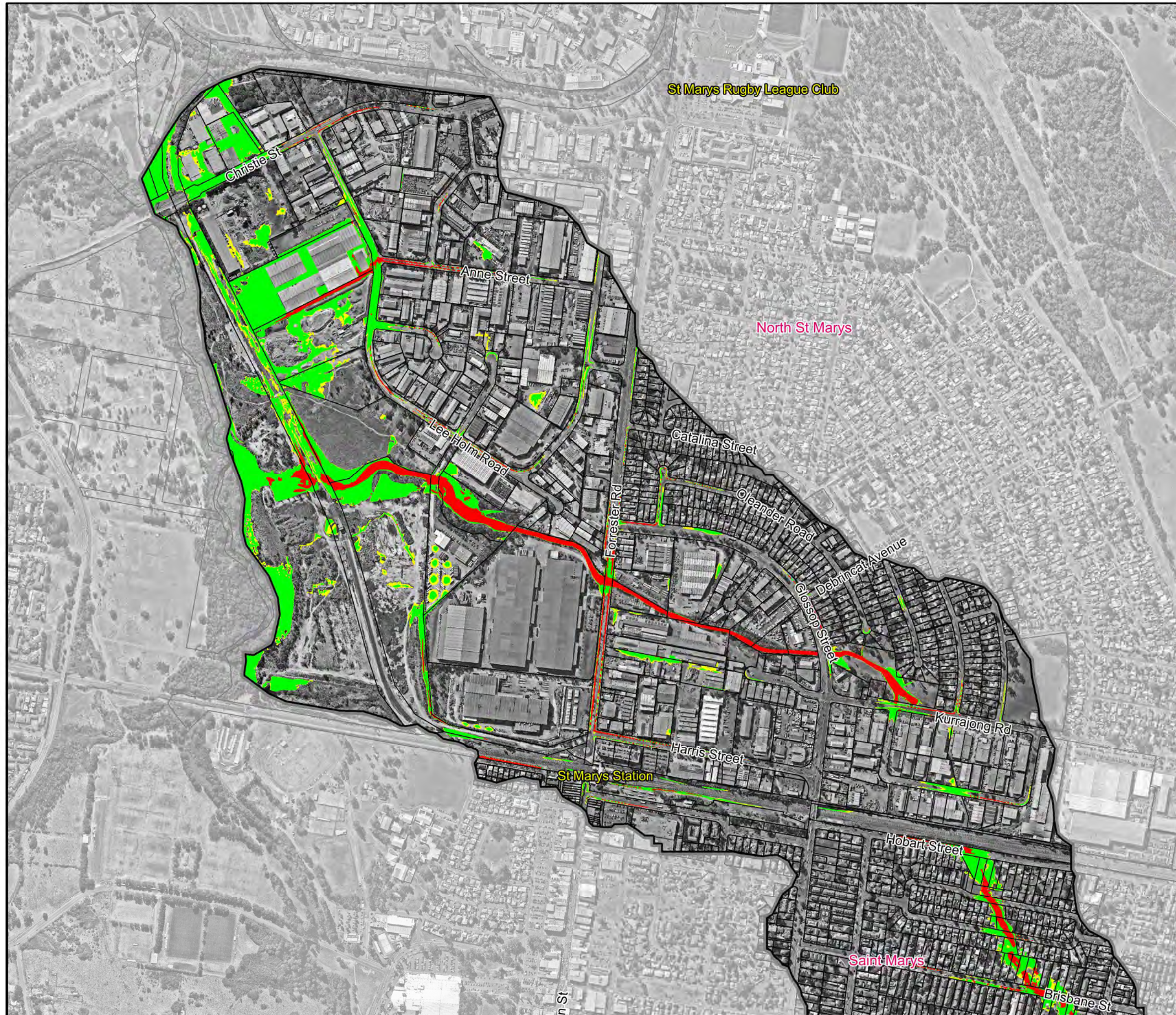
Figure 38.2 Hydraulic Categories for the 5%AEP
