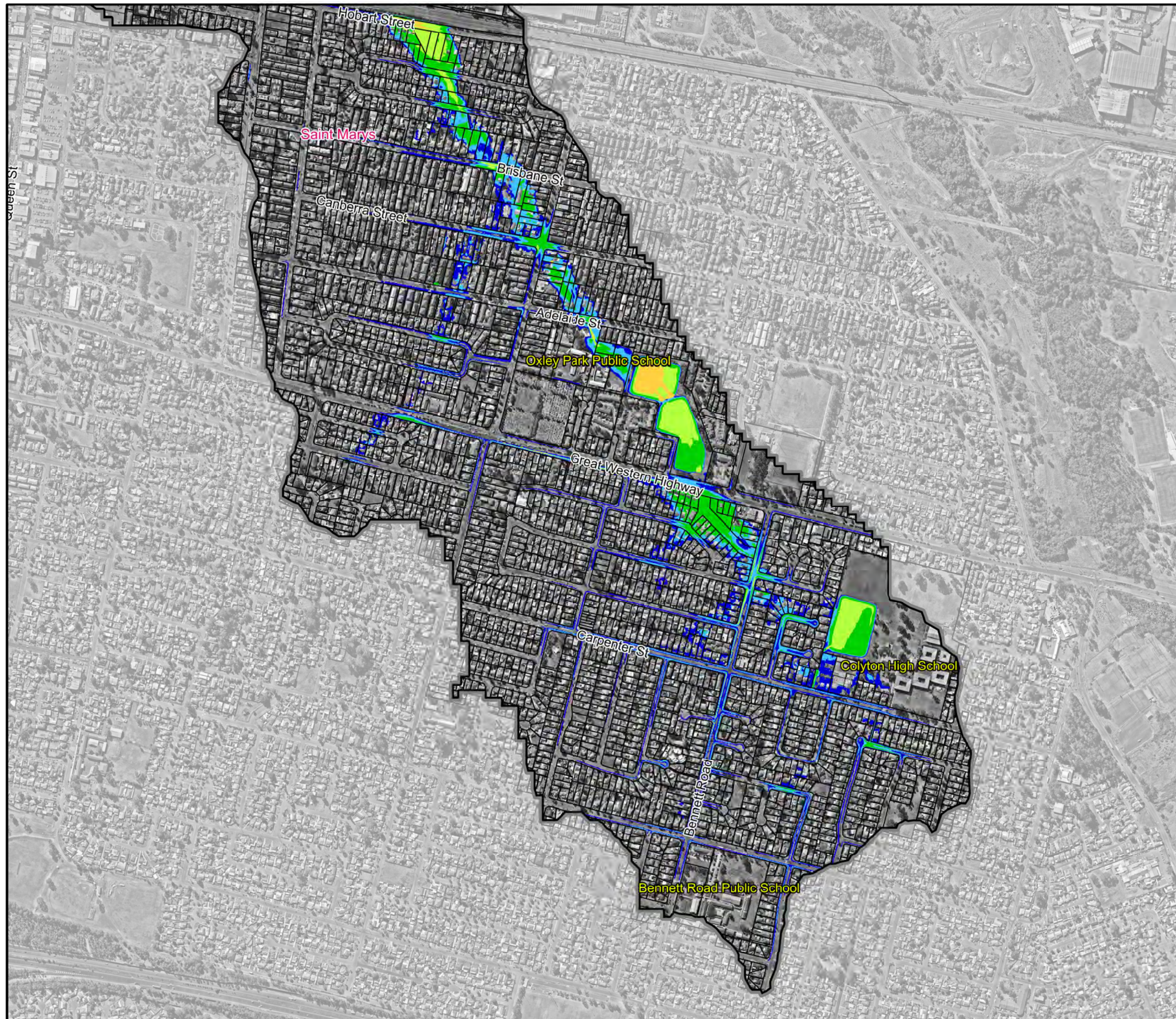
Figure 36.1 Flood Hazard for the 0.2% AEP Flood
