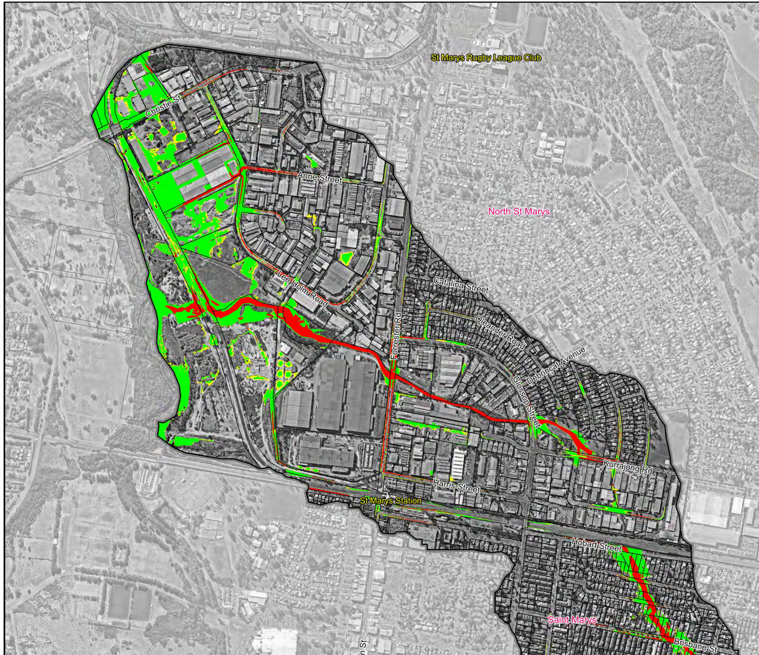
Figure 39.2 Hydraulic Categories for the 1%AEP
